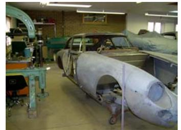
the right door framework, which was beyond repair, and rebuilt the driver's side door frame. The door skins will be fabricated and installed after the front fenders are repaired and permanently reinstalled.
