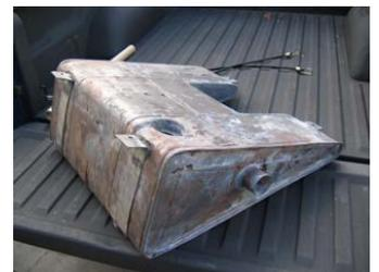
A rusty original steel tank, full of holes; new tanks patterned after this.
