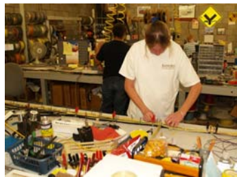
Each new harness is crafted one-at-a-time by hand according to the original pattern
