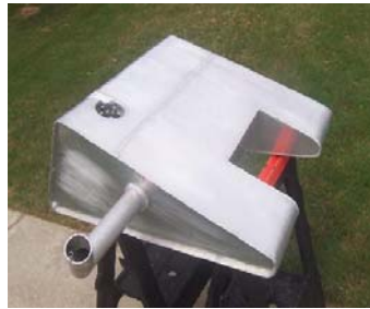
Repro tank is made of aluminum and follows the pattern & contours...
