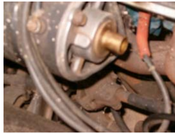
Detail of brass fitting heat-shrunk into the back of the generator
