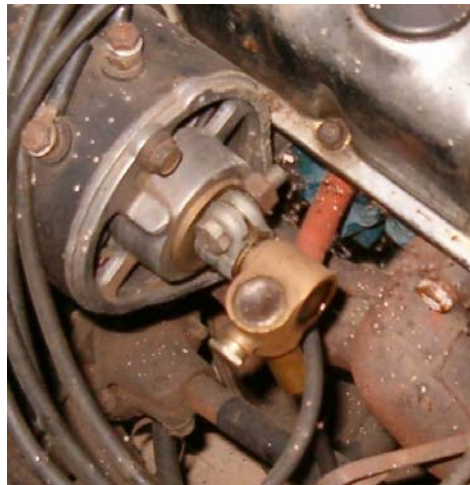
Photo of completed installation; note cable exiting down from angle drive. That'll get hot!
