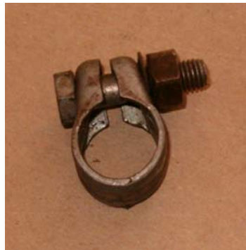
Here's the Fiat 600 tie rod clamp used to couple the angle drive to the brass fitting
