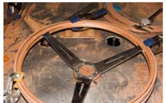
what I refer to as a full wrap, with wood covering all four sides of the rim. These type wheels naturally needed no rivets to help secure the wood to the inner metal rim because the wood fully encases the metal rim. And
